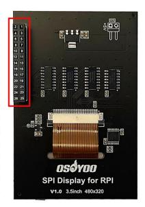
The pins marked as "NC" below indicate that the pins are not occupied by the LCD and can be used by the user for other applications.
