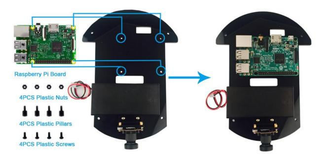
STEP12. Before install the top chassis as follows, you need to plug the battery box into model pi motor driver, then connect the Raspberry Pi board to PCA9685 compatible module and model Pi motor driver board, Lastly, connect 5 pcs tracking sensors to raspberry pi as follows.
