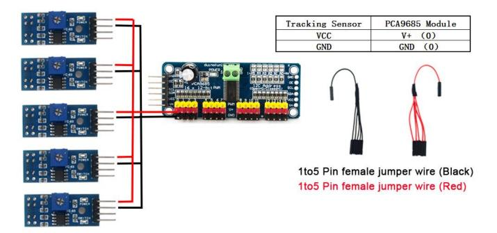
STEP8. Install the model pi motor driver board as follows. Then connect PCA9685 compatible module to motor driver board via 4pin and 2 pin cable. Meanwhile, connect the voltage meter to motor driver board via 3pin cable.
