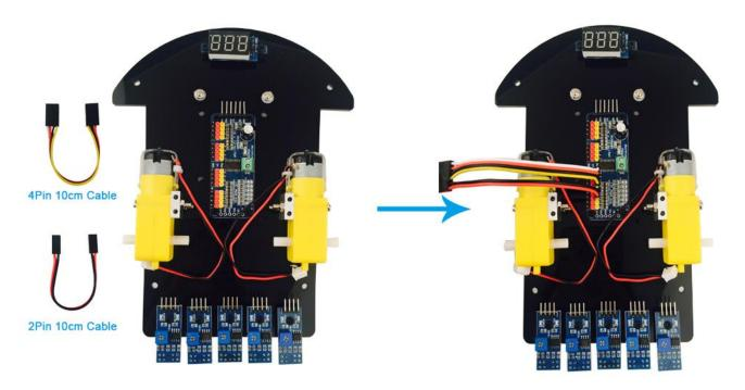
STEP7. Plug the 2 PCS 1 pin to 5 pin female to female cable (Black and Red) into PCA9685 compatible board as follows.
